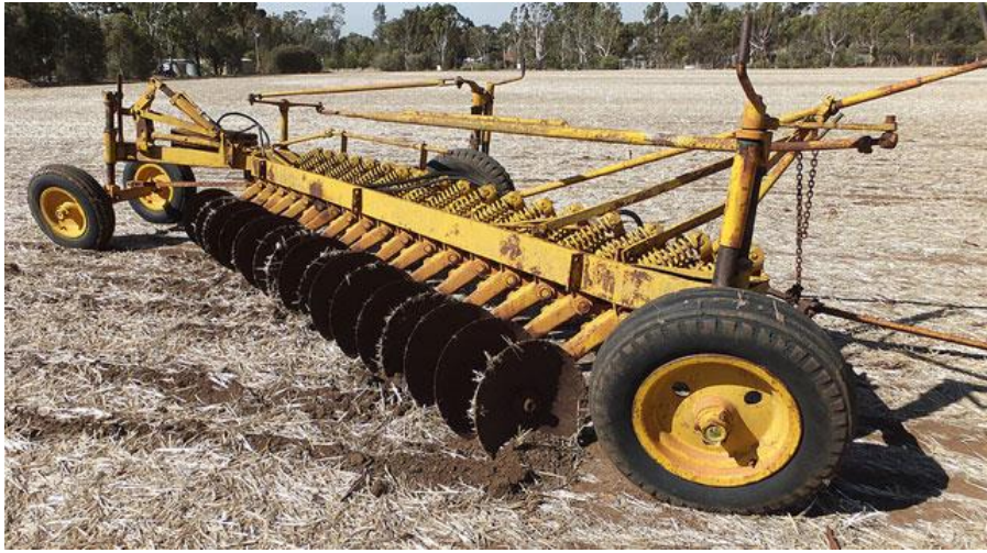
Figure 7 - A similar one-way chamberlain plough to the one used at Tony Whites. Photo: Alton Materials
