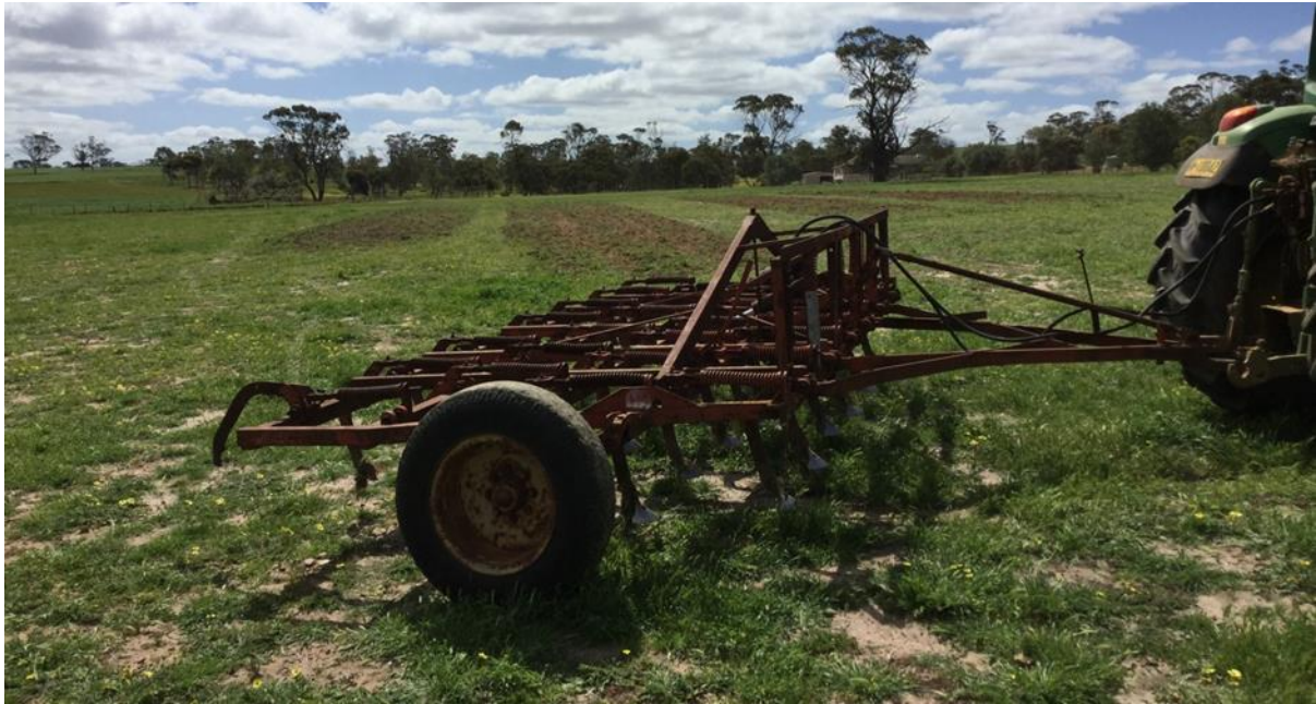
Figure 5: Scarifier bar used at Jeremy Lefroys and Richard Humphrys. Photo: Wes Lefroy
